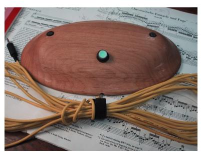
Features: Pilot light is also batterylife indicator. Protection circuitry prevents damage from wrong insertion of batteries.
